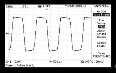
Output section clipping, Main Gain on 10
